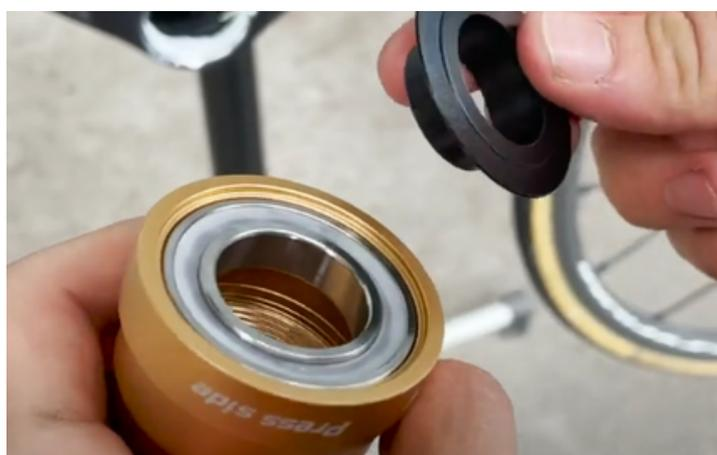
**By using a press, press the right cup (press side) into the frame, on drive side.**
